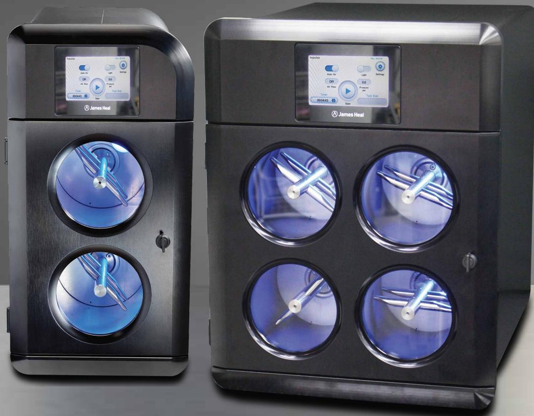
Our Impulse range, available in 4 or 2 chamber models, are the only instruments that offer interchangeable impellers and greatly improved sample rotation throughout the test to give reliability, accuracy and flexibility.
