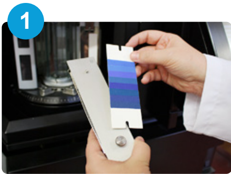
The mask or cover is placed upon the specimen and firmly positioned using the notches on the Tri-sided holder.
