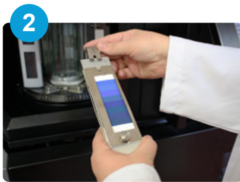
After a mid-test visual assessment these guides ensure the mask or cover is placed back in exactly the same position.
