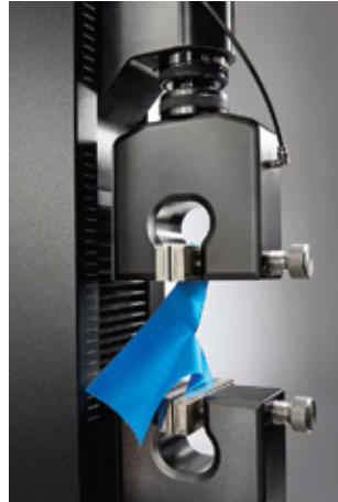
Tear Strength Test (T27)
