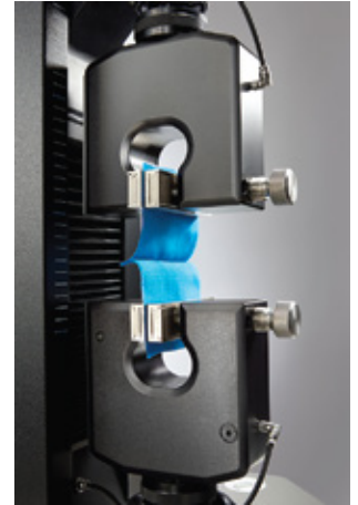
Seam Slippage Test (T27)
